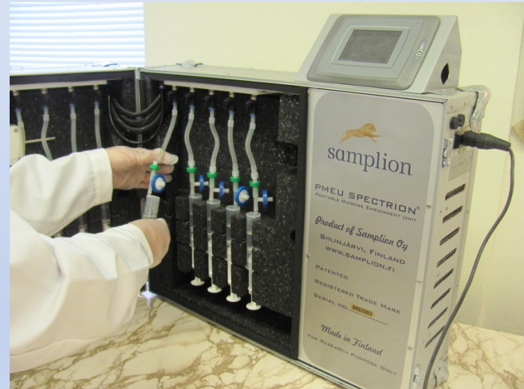
Fig. 2. PMEU Spectrion® in operation with the sampling and cultivation syringes. On the right top the control unit with wireless and Ethernet connections.
