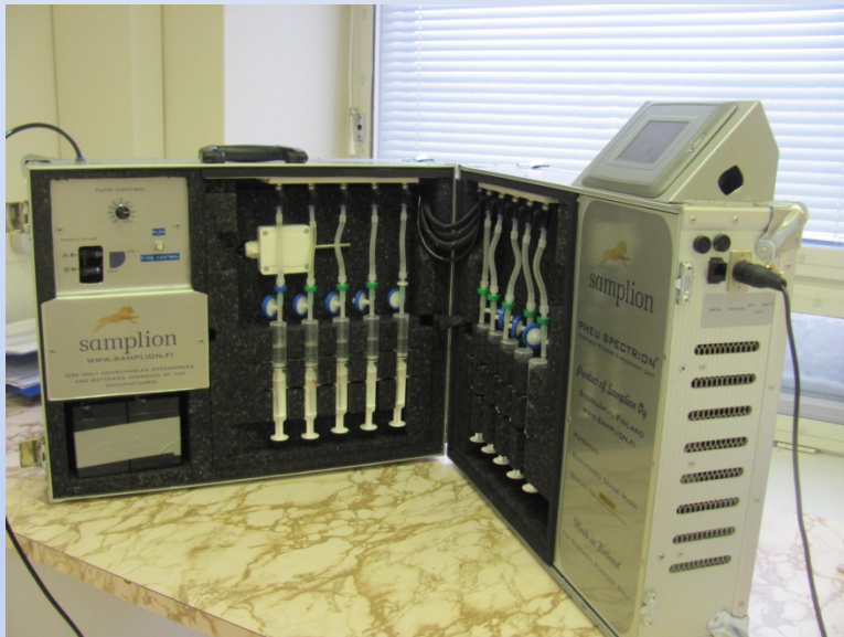
Fig. 2. PMEU Spectrion® in operation with the sampling and cultivation syringes. On the right top the control unit with wireless and Ethernet connections.
